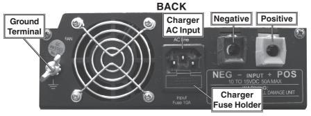
**WARNING!** Risk of Fire! The positive battery terminal connection must be the LAST connection and must be done with the inverter's switch off.
